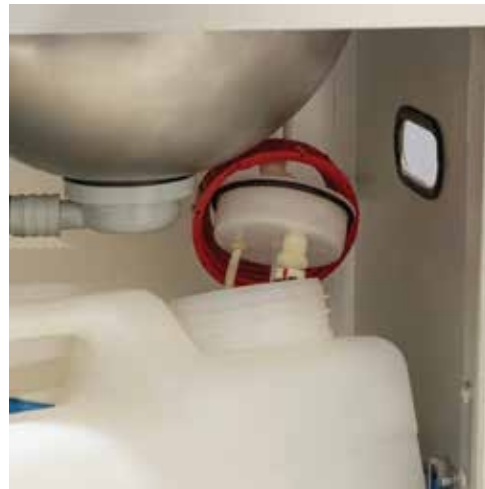
Picture 15. Cap of the clean water canister unscrewed.
