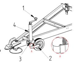
Figure 2: support wheel fixed in the upper position.
