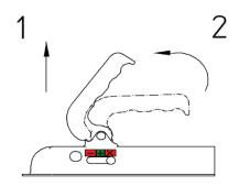
Figure 3: uncoupling the coupling device.
