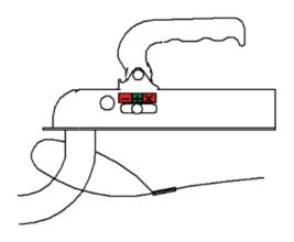
Figure 1: locked coupling device.
