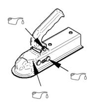
Figure 4: coupling device areas requiring lubrication.
